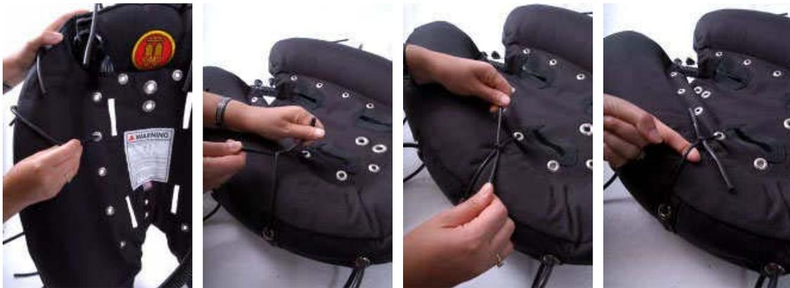
Step Six: Now that all the knots are tied, pull each of them around so that it is safely tucked near the backside of each inner grommet (tank side/no-label side).
