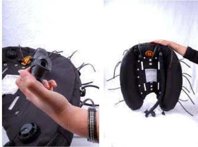
Step Five: With the BC facing you (label side towards you), string one end of each retraction band through their corresponding inner grommet (grommet directly to the right of the outer grommet set you are stringing). Be sure you string the band from the front to the back and tie a square knot on the no-label side. Be sure the knot is snug. Snug is defined as being able to work your finger between the band and BC with little effort. Repeat this process for all 12 grommet sets.
